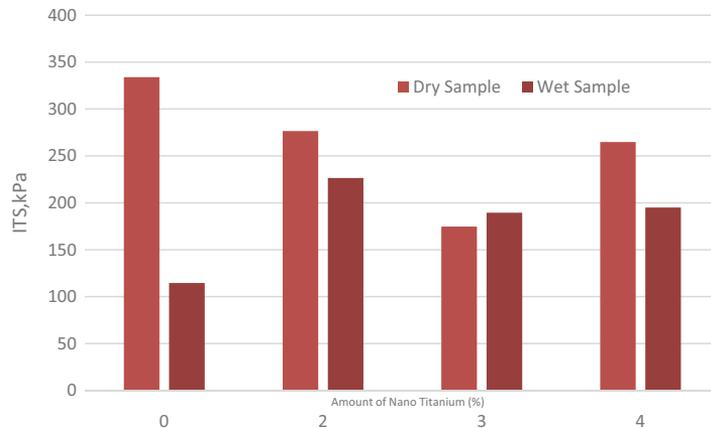
Fig. 4. ITS Value vs Amount of Nano Titanium
