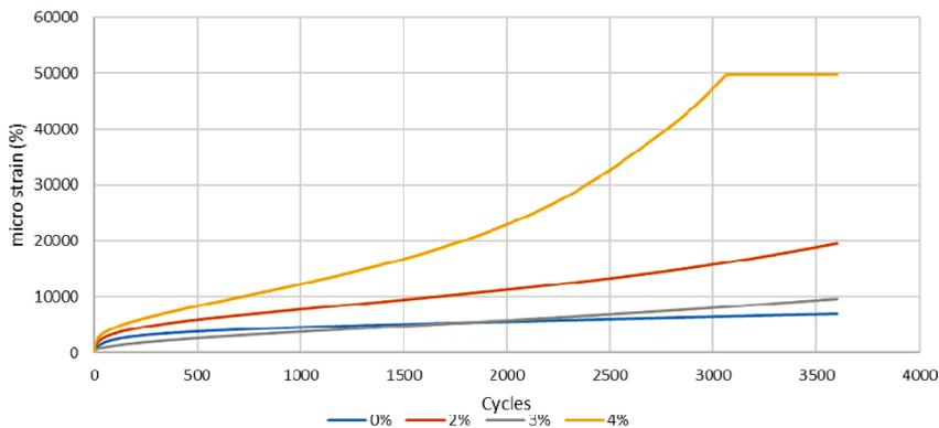
Fig. 3. Strain Values for each modified SMA Specimen
