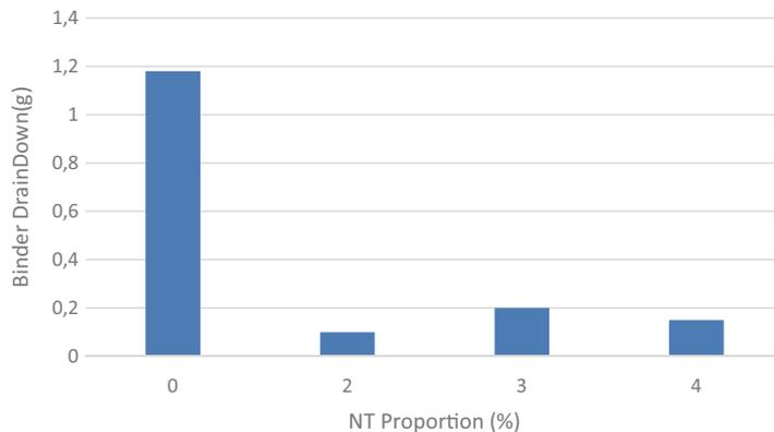
Fig. 6. Binder drain down vs Nano Titanium
