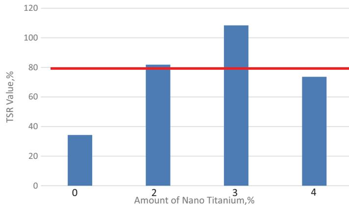
Fig. 5. ITSR Value (%) vs Amount of Nano Titanium (%)
