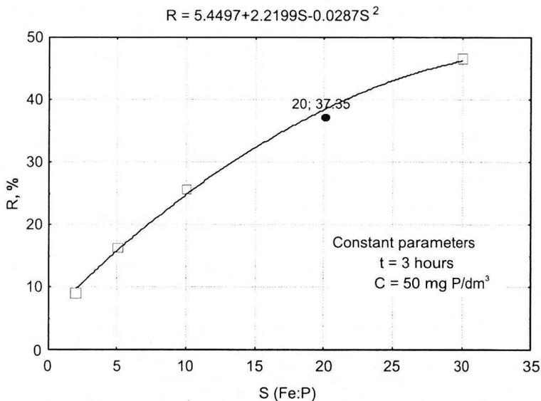
Fig. 5. Influence of Fe:P ratio (S) on average percentage removal of orthophosphates from model solution (R), pH  $\approx$  7
