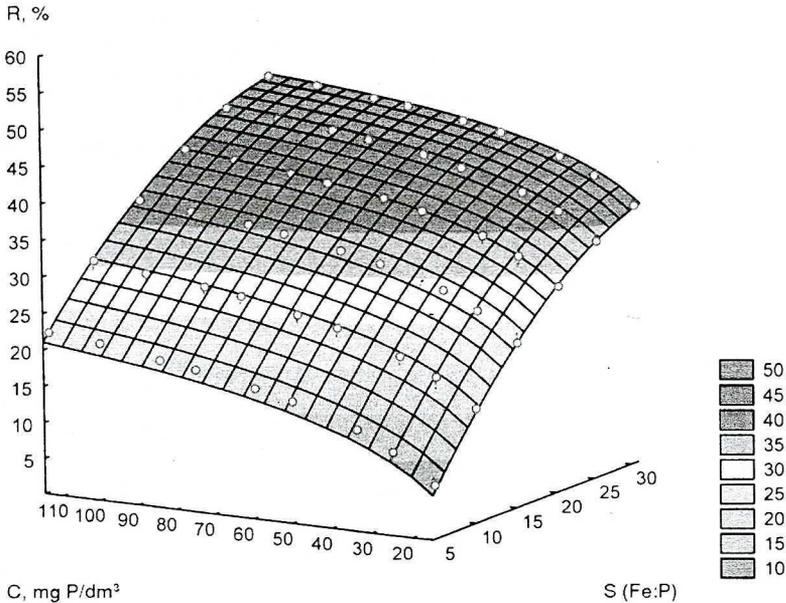
Fig. 7. Influence of initial concentration (C) and Fe:P ratio (S) on percentage removal of orthophosphates (R). Reaction time of 3 hours,  $\text{pH} \approx 7$
