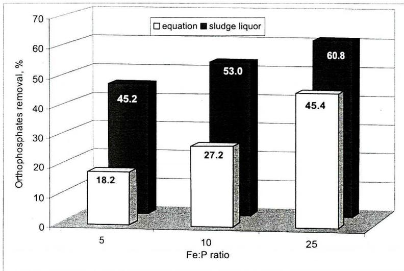
Fig. 9. Percentage value of orthophosphates removal from sludge liquor and value calculated based on equation for model solution depending on value of Fe:P ratio. Initial concentration of 76.6 mg P-dm<sup>-3</sup>, reaction time of 3 hours, pH ≈ 7
