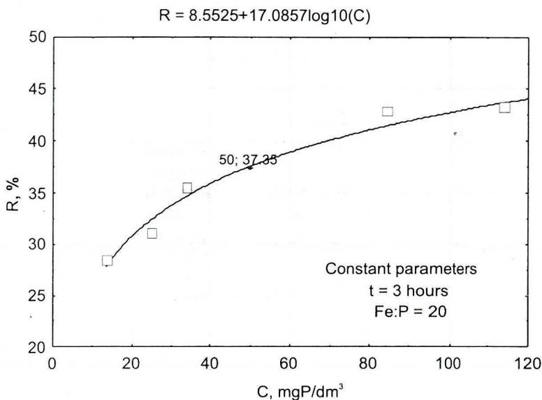
Fig. 6. Influence of initial concentration of orthophosphates (C) on average percentage removal of orthophosphates from model solution (R), pH  $\approx$  7
