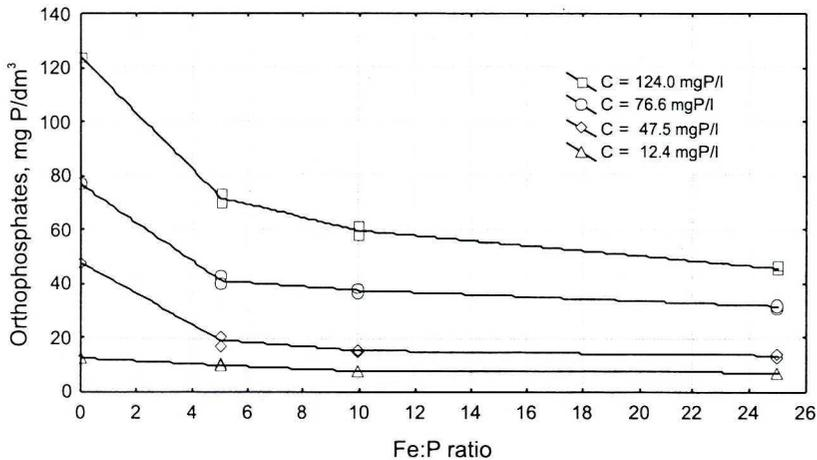
Fig. 8. Removal of orthophosphates from sludge liquor in function of initial concentration (C) and Fe:P ratio value. Reaction time of 3 hours, pH ≈ 7
