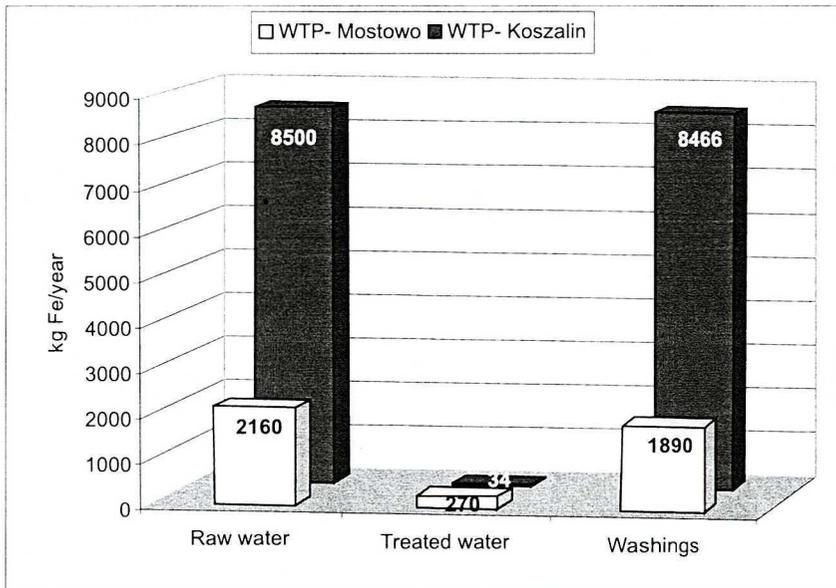
Fig. 3. Average amount of iron in raw water, treated water and washings in tested plants
