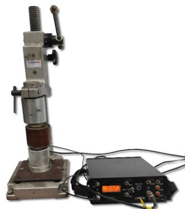
Fig. 3. Research set-up for ultrasound tests of pathways of bonding moulding sands with chemical binders
