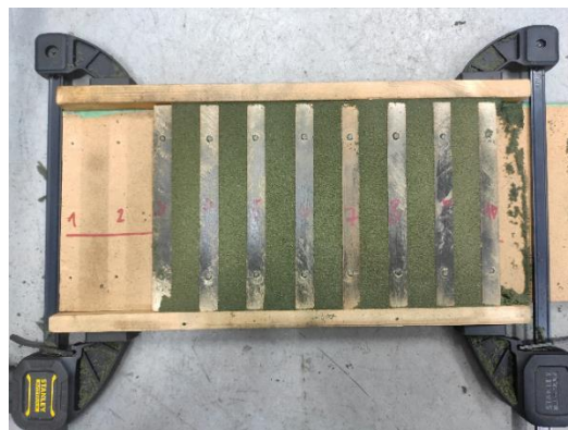
Fig. 4. Sampler for making shaped elements intended for measuring the deflection angle in the bend test
