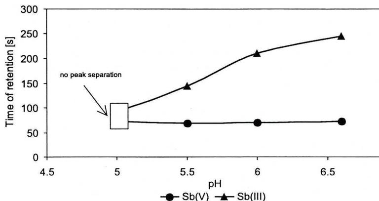
Fig. 2. Effect of the eluent (ammonium tartrate) pH on retention time of Sb(V) and Sb(III) species (eluent concentration  $400\text{ mmol}/\text{dm}^3$ ; for standard  $250\text{ ng}/\text{cm}^3$  of each form of antimony)
