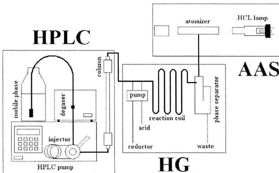
Fig. 1. Schematic diagram of the HPLC-HG-AAS instrumentation
