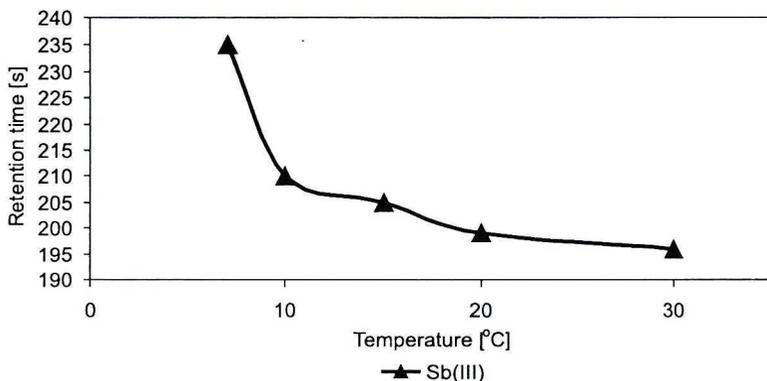
Fig. 4. Effect of the column temperature on retention time of Sb(III), retention time of Sb(V) is constant (eluent 400 mmol/dm<sup>3</sup>, pH 6.6–6.7; for standard 250 ng/cm<sup>3</sup> of antimony)
