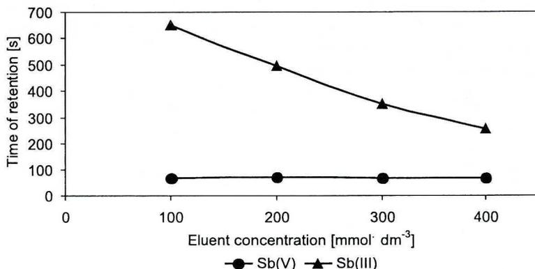
Fig. 3. Effect of the eluent concentration (ammonium tartrate) on retention time of Sb(V) and Sb(III) species (eluent pH 6.6–6.7; for standard 250 ng/cm<sup>3</sup> of each form of antimony)
