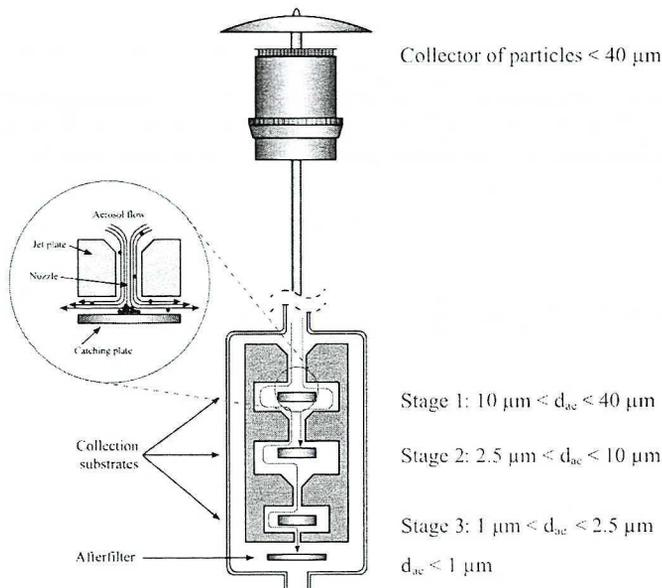
Fig. 3. The Dekati PM-10 working principle
