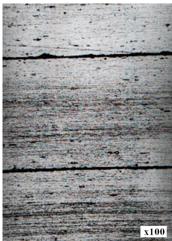
Fig. 6. Metallographic analysis of the hot strip rolling, thickness: 0.25 mm
