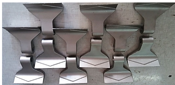
Fig. 9. Manufactured casts of RM4 mulchers
