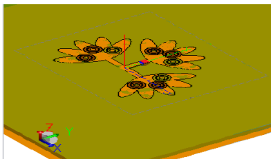
Fig. 18. Fig. 12. 3D geometrical view with SRRs
