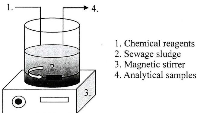
Fig. 1. Scheme of the experimental stand
