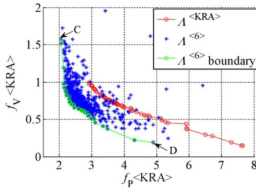
Figure 11: Comparison of the six-dimensional set of compromises  $\Lambda^{<6>}$  and its two-dimensional boundary  $\Lambda^{<6>}$  boundary with the two-dimensional set of compromises  $\Lambda^{<KRA>}$  on the plane  $f^{<KRA>}$
