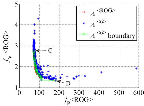
Figure 10: Comparison of the six-dimensional set of compromises  $\Lambda^{<6>}$  and its two-dimensional boundary  $\Lambda^{<6>}$  boundary with the two-dimensional set of compromises  $\Lambda^{<ROG>}$  on the plane  $f^{<ROG>}$
