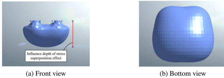
Fig. 7. Peak dynamic stress iso-surface ( \delta_{zz} = -6 kPa)
