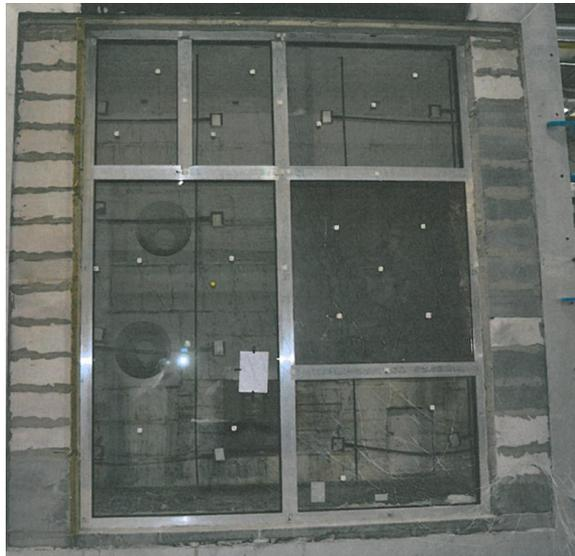
Fig. 4. View of the MB-118/EI system partition test element (partition G). Source [11]
