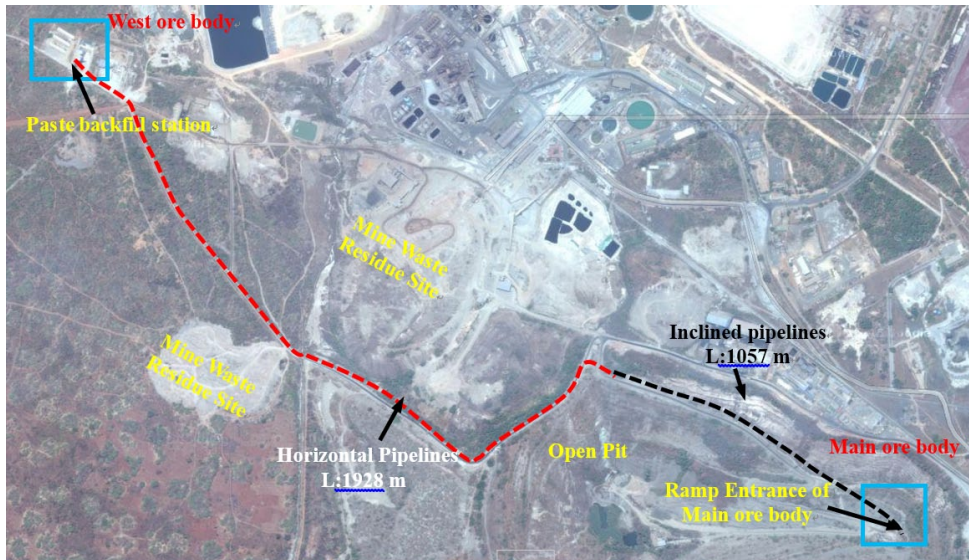
Fig. 13. Surface conveying line of paste slurry for major ore body
