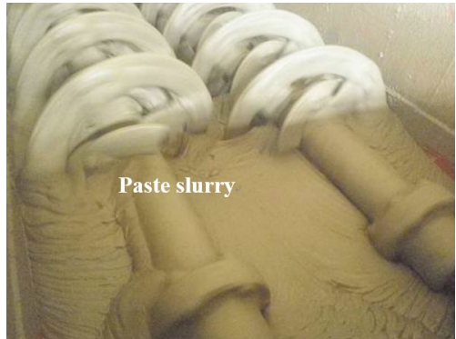
Fig. 6. Paste slurry in mixer (wt.70.4%)
