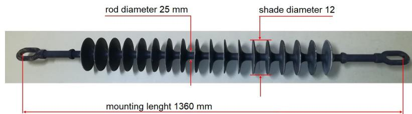
Fig. 2. Composite insulator removed from the line after 35 years of operation
