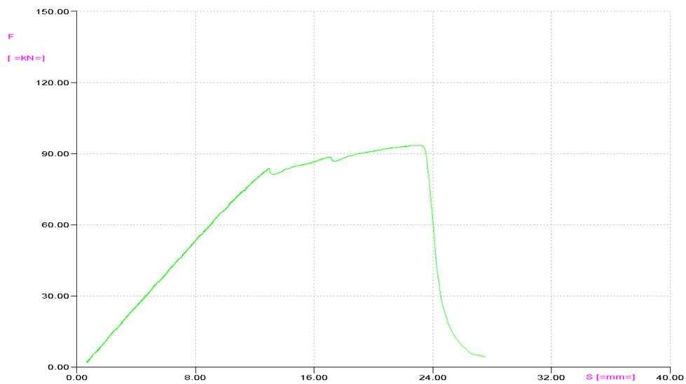
Fig. 6. Relationship between elongation and tensile load for insulator from Fig. 2 in mechanical strength test under static load
