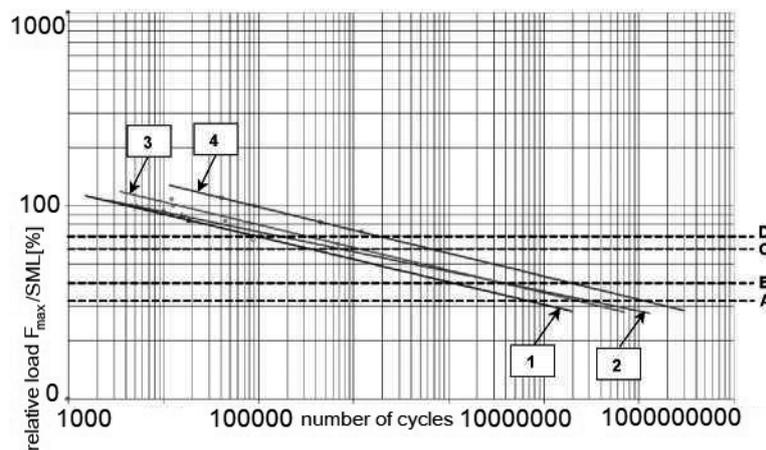
Fig. 8. Fatigue characteristics of composite insulators, determined for selected values of amplitudes of cyclic load changes (logarithmic scale on both axes):
