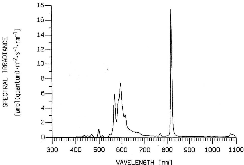
Fig. 3. Spectral irradiance in the range of 300–1100 nm inside the exposure chamber (measurement at 2 nm intervals with LI-1800 LI-COR USA) provided by Philips SOD-4 Agro 400W lamps
