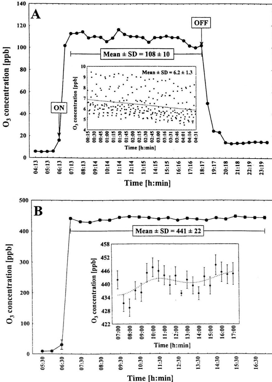
Fig. 4. An example of the dial O<sub>3</sub> concentration in the exposure chamber (each point presents mean value from 30 estimations): A – at O<sub>3</sub> concentration 110 ppb (inside – changes in O<sub>3</sub> concentration in external air); B – at O<sub>3</sub> concentration 450 ppb (inside – fluctuation of O<sub>3</sub> during the fumigation in enlargement)
