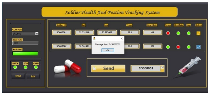
Fig. 17. The IGUIM for SHAPTS when a message is sent to soldier SD1 correctly
