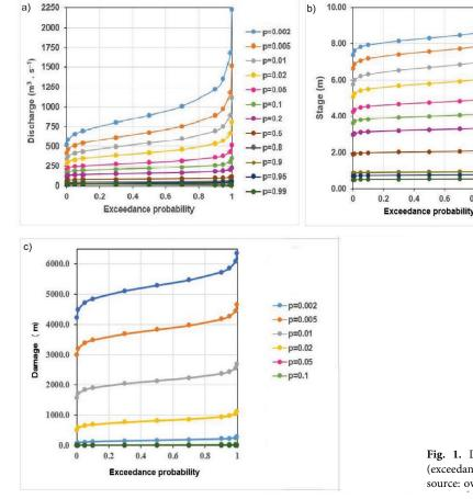
Fig. 1. Distribution function with different return period (exceedance probability - p): a) discharge, b) stage, c) damage; source: own study
