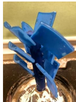
Fig 1. Wax system: patterns assembled on a “tree”
