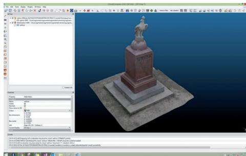
Fig. 4. Result of surface reconstruction in CloudCompare
