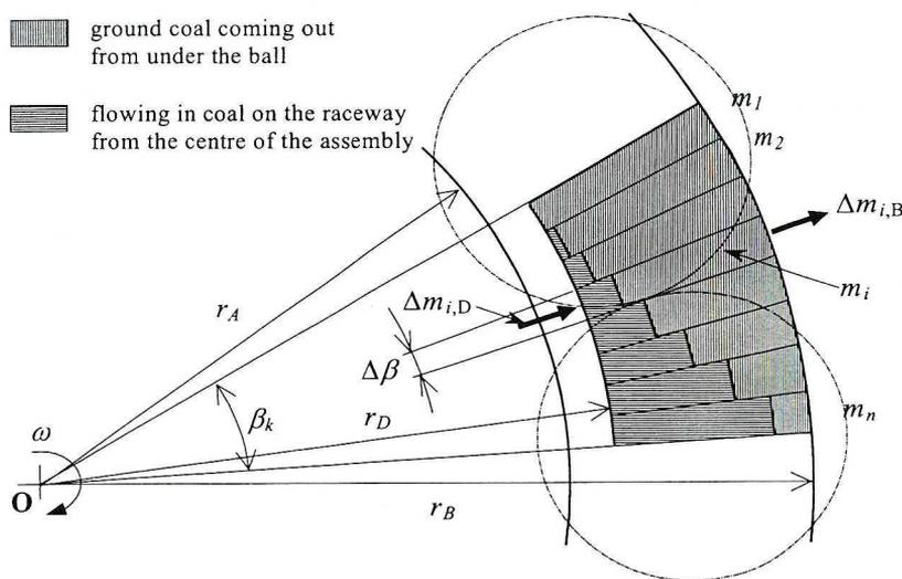
Fig. 10. Flow visualization of coal on the active arc of the raceway
