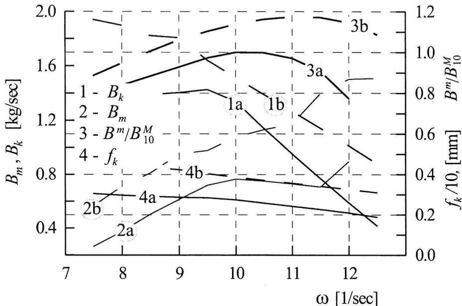
Fig. 13. The influence of the number of balls on the characteristic calculated values of the assembly for:  $\alpha_A = \alpha_B = 45^\circ$ ,  $s_k = 125$  kPa, a -  $z_k = 10$ , b -  $z_k = 6$
