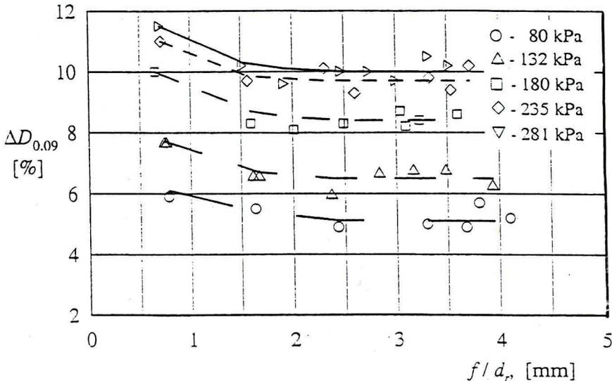
Fig. 4. The effect  $\Delta D_{0.09}$  – layer thickness relations at different unit-pressures under the roller  $d_r = 150$  mm, primary crushing
