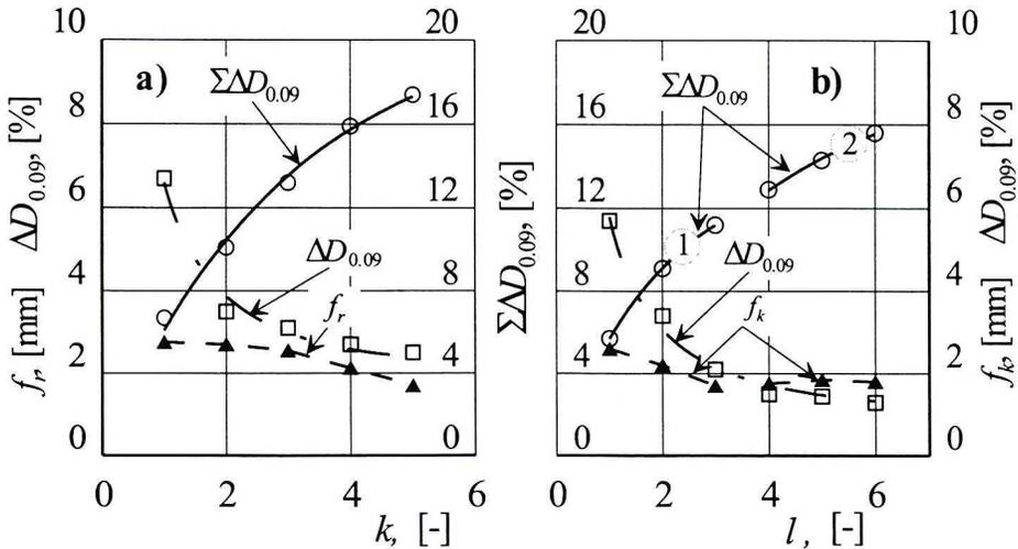
Fig. 6. The influence repeated crushing on the effect and layer thickness. a) roller –  $d_r = 150$  mm,  $s = 231$  kPa,  $f_0 = 8$  mm, b) ring-ball assembly –  $d_k = 100$  mm,  $s_k = 115$  kPa,  $\omega = 8.2$  1/sec
