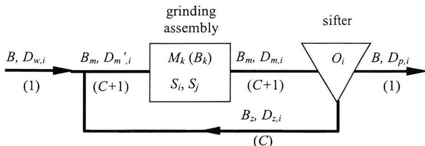
Fig. 1. Circuit model of grinding with classification
