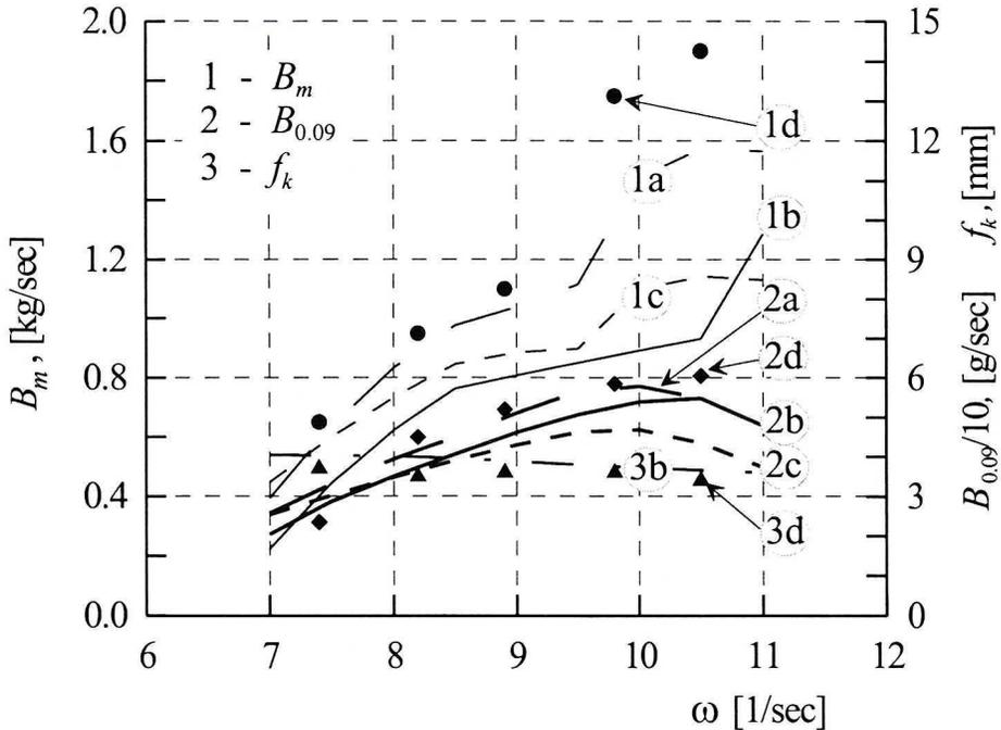
Fig. 11. Flow and efficiency of a grinding assembly without ventilation for:  $z_k = 7$ ,  $\alpha_A = \alpha_B = 45^\circ$ ,  $s_k \approx 68$  kPa,  $\mu = 0.40$ ,  $\mu_w = 0.65$ ; a – the effect of the stream in the direction  $\alpha - n_{\alpha,D}$  and  $f = \text{constant}$ ; b – according to the modelling conditions and  $f = \text{constant}$ ; c – exemplary linear distribution of the layer; d – experimental results
