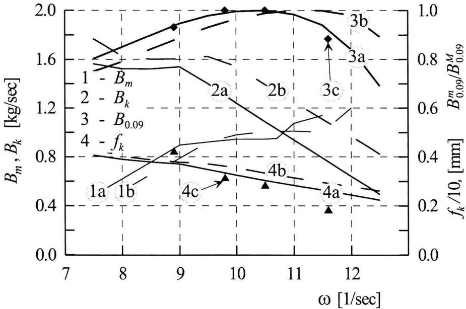
Fig. 12. Influence of the friction factors for:  $z_k = 7$ ,  $\alpha_A = \alpha_B = 45^\circ$  i  $s_k = 116$  kPa: a -  $\mu = 0.45$  i  $\mu_w = 0.70$ ; b -  $\mu = 0.50$  i  $\mu_w = 0.75$ , c - experimental results
