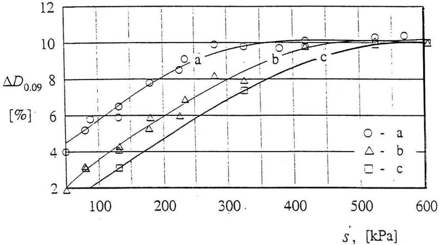
Fig. 5. The influence of pressure on the grinding effect of the size class  $0 \div 2$  mm by  $f/d_r = 4\%$ . a – primary crushing, b – secondary crushing after screening of the size class  $0 \div 0.2$  mm (dust), c – third crushing after repeated screening of dust
