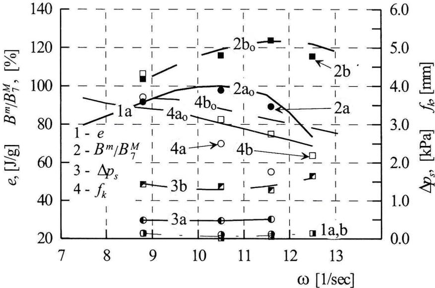
Fig. 15. The influence of the raceway slope on the efficiency of the mill for:  $z_k = 7$ ,  $s_{k,1} = s_{k,2} = 157$  kPa, a -  $\alpha_A = \alpha_B = 45^\circ$ , b -  $\alpha_A = 30^\circ$ ,  $\alpha_B = 60^\circ$ .
