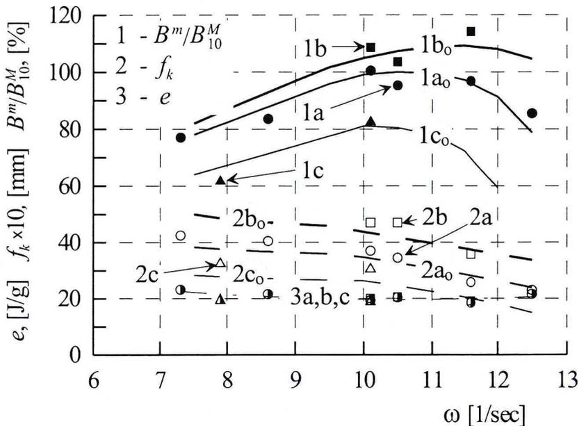
Fig. 14. The influence of the number of balls on the efficiency of test mill for: a -  $z_{k,1} = 7$ , b -  $z_{k,2} = 10$ , c -  $z_{k,3} = 14$ ,  $s_k \approx 70$  kPa. Subscript "o" - calculations
