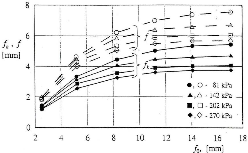
Fig. 3. The thickness of the drawn-in layer as a function of its initial thickness ( $d_r = 125 \text{ mm}$ ), (Pulling conditions of the coal layer)
