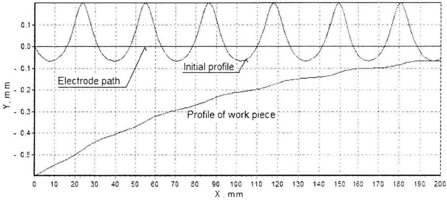
Fig. 5. The profiles from software screen ( $R_0 = 10$  mm,  $a_0 = 0.6$  mm,  $\nu = 0.3$ )
