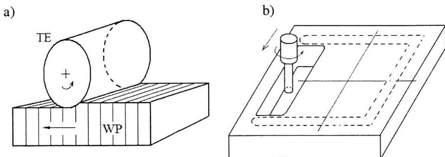
Fig. 1. Example of machining using rotating tool electrode (TE). a) Machining of pocket samples; b) Contouring by REDM
