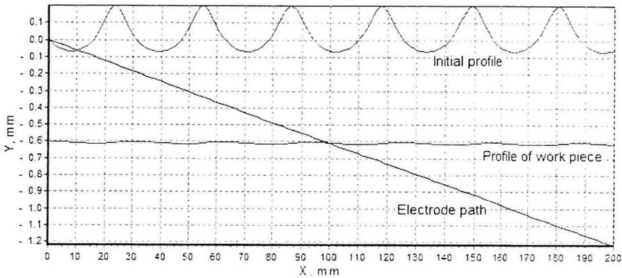
Fig. 6. Surface profile and tool path at REDM with compensation of tool wear ( $R_0 = 10$  mm,  $a_0 = 0.6$  mm,  $\nu = 0.3$ )
