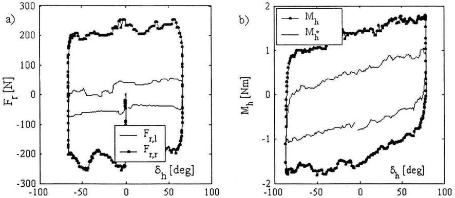
Fig. 11. a) The reaction forces in both tie rods versus the steering angle. Steering system with free rotating handwheel is moved from its initial position by exerting a moment of forces  $M_z$  at the right wheel. b) Comparison of the resistant torque  $M_h$ , measured at the handwheel, and  $M_h^*$  determined using formula (9). Suspension in the design position
