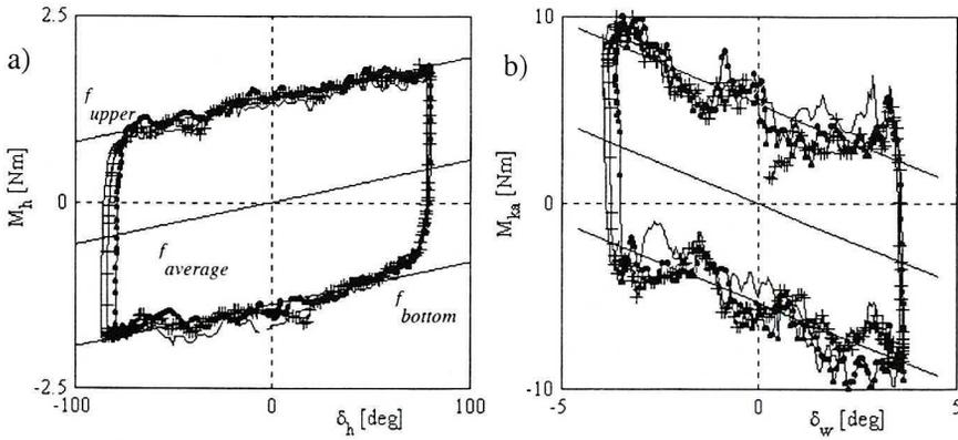
Fig. 10. Exemplary characteristics of a) steering torque vs. steering angle, and b) torque with respect to kingpin axis vs. left wheel steer angle for a sinusoidal steering angle excitation ( $f = 0.1$  Hz). Front wheels supported at the rotating plates. Results of three trial repetitions are superimposed
