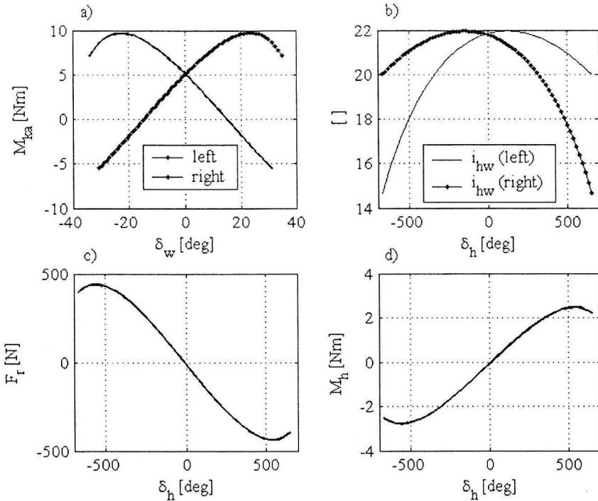
Fig. 5. Quasi-static characteristics of load transmission from the road wheels to the steering wheel resulting from the wheel normal force only (friction neglected): a) torque with respect to the kingpin axes versus steer angle, b) the overall kinematical ratio of steering system for left and right wheels, c) the steering rack force, d) torque at the steering wheel versus angle of steering wheel
