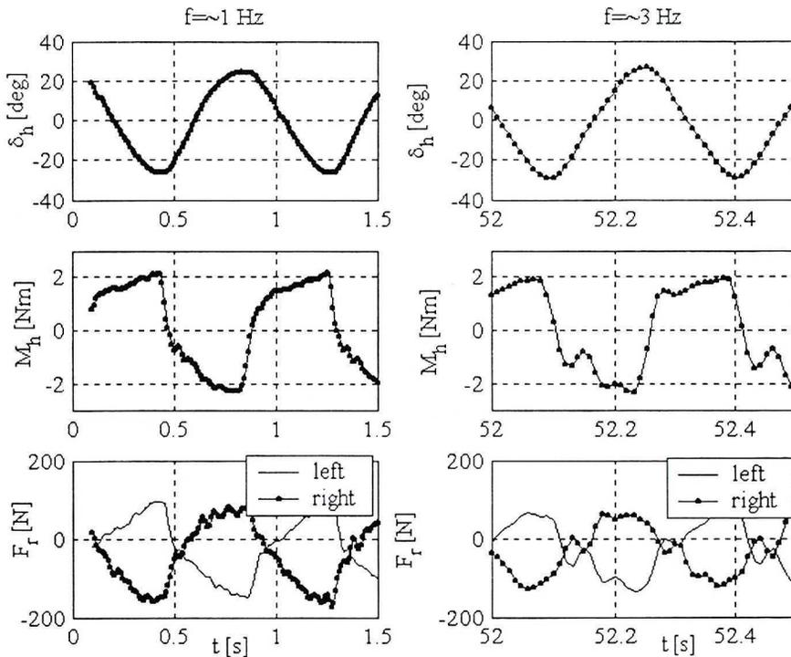
Fig. 7. Time responses of the steering system. Top: harmonic changes of the steering angle  $\delta_h$ . Center: resistance torque at the handwheel  $M_h$ . Down: axial forces  $F_r$  in the tie rods. Frequency  $f \approx 1$  Hz (a) and  $f \approx 3$  Hz (b). Front wheels supported at the rotating plates
