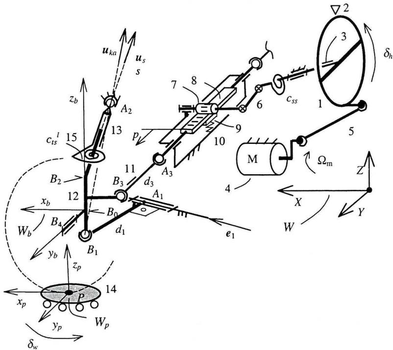
Fig. 2. Kinematic scheme of the front strut suspension with rack-and-pinion steering system in trailing configuration, and road wheels supported on rotational plates of the test stand. Left side is shown only
