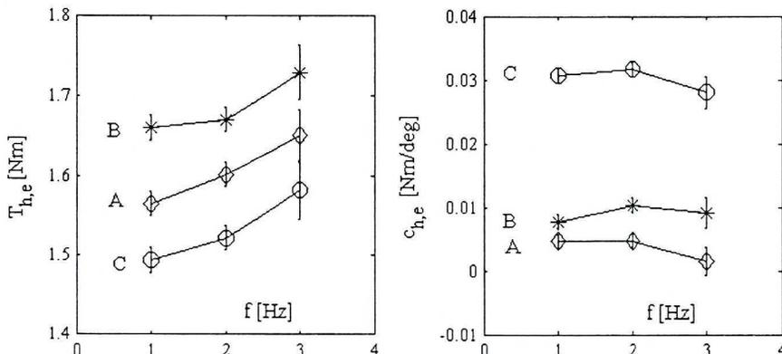
Fig. 13. Estimates of the model parameters reduced to the handwheel. Influence of the pseudo-sinusoidal excitation frequency and different load conditions (A, B, C) is presented
