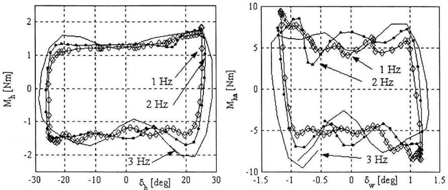
Fig. 12. Steering torque vs. steering angle (left), and torque relative to kingpin axis vs. left wheel steer angle (right) for a sinusoidal steering angle excitation with frequency  $f = 1, 2,$  and  $3$  Hz. Front wheels supported at the rotating plates,  $F_z^F = 2.50$  kN
