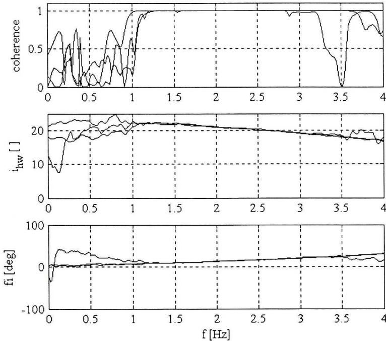
Fig. 8. Frequency domain relationships (coherence, module and phase shift) between input signal – rate of the wheel steer angle and output signal – rate of the steering angle for a pseudo-sinusoidal excitation with an amplitude of 25 deg. Front wheels supported at the rotating plates. Results of three trial repetitions are superimposed
