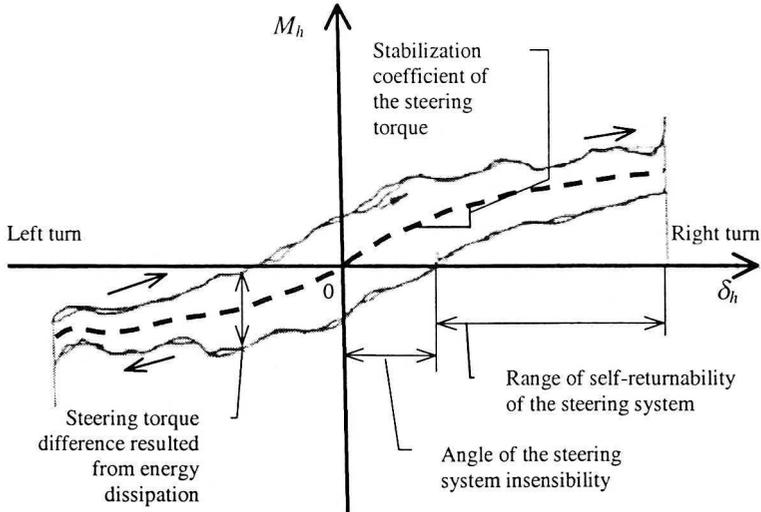
Fig. 1. Typical characteristics of the steering torque (measured at the hand-wheel) as a function of the steering angle for a car taking a slalom maneuver with a constant speed [5]
