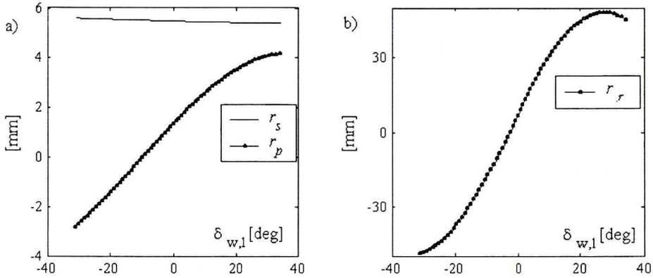
Fig. 4. Variation of:  $r_s$  – roll radius,  $r_p$  – arm of the wheel normal force (a), and  $r_\tau$  – castor offset (b) versus road wheel steer angles for a left wheel. Suspension is in the design position
