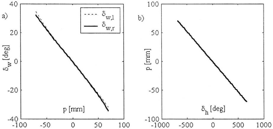
Fig. 3. a) Steer angles of the road wheels  $\delta_{w,l}$  and  $\delta_{w,r}$  (left and right) versus the steering rack displacement  $p$ ; b)  $p$  versus steering angle  $\delta_h$ . Suspension is in the design position
