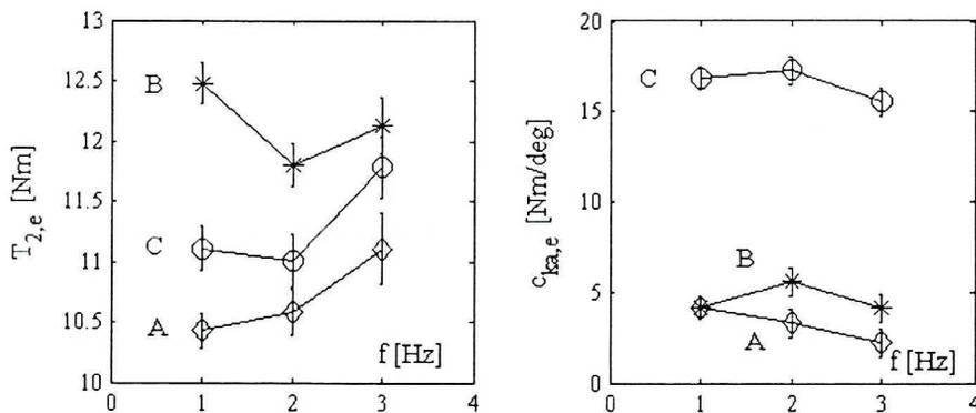
Fig. 14. Estimates of the model parameters reduced to the kingpin axis. Influence of the pseudo-sinusoidal excitation frequency and different load conditions (A, B, C) is presented
