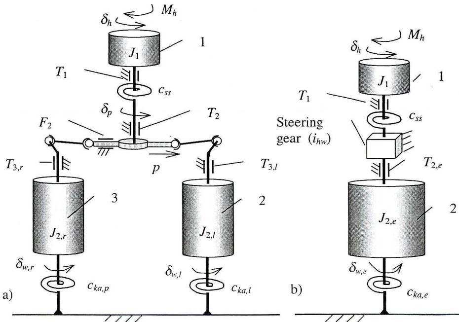
Fig. 6. The models of the steering system with: a) three lumped masses, b) two lumped masses valid for small amplitudes of steer angle changes
