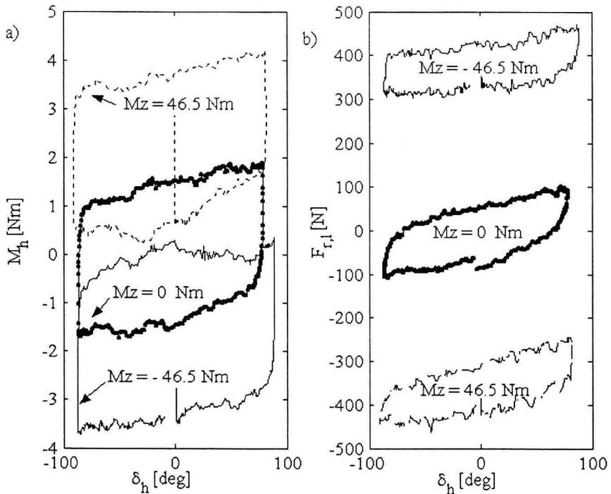
Fig. 9. a) The handwheel resistant torque and b) reaction force in the left tie rod versus the steering angle. Quasi-static sinusoidal excitation of the steering angle. The front wheels are supported at rotating plates, and the left one is loaded by a constant aligning torque  $M_z$  (with values:  $-46.5$ ,  $0$ ,  $46.5$  [Nm]). Suspension in the design position
