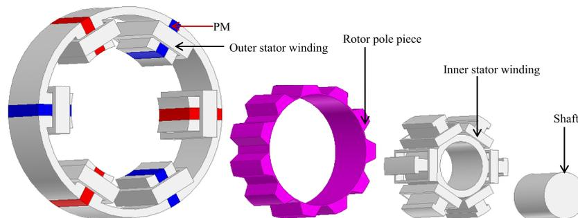
Fig. 1. Exploded view of Machine 1 [11]
