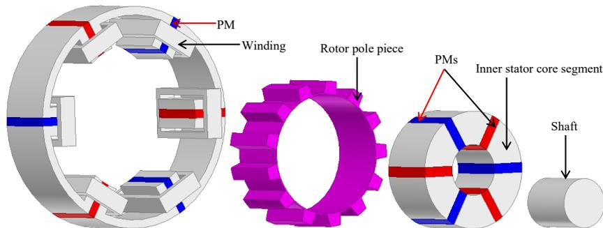
Fig. 3. Exploded view of Machine 3
