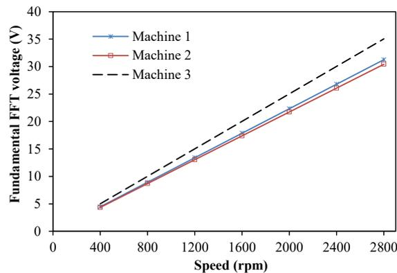
Fig. 5. Variation of fast Fourier transform (FFT) induced-EMF with speed, 2D-FEA
