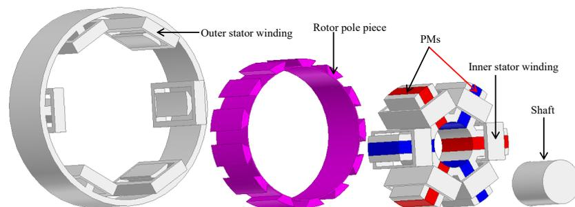
Fig. 2. Exploded view of Machine 2
