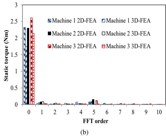
Fig. 6. Comparison of static torque at  $I_A = 15$  A and  $I_A = 2I_B = -2I_C$ , 400 rpm: waveforms (a); spectra (b)
