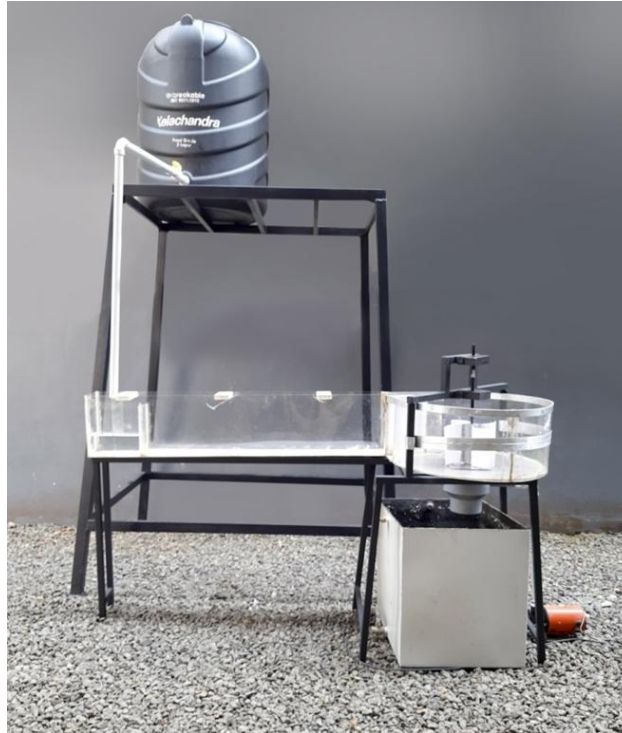
Fig. 4. Gravitational Water Vortex experimental set up
