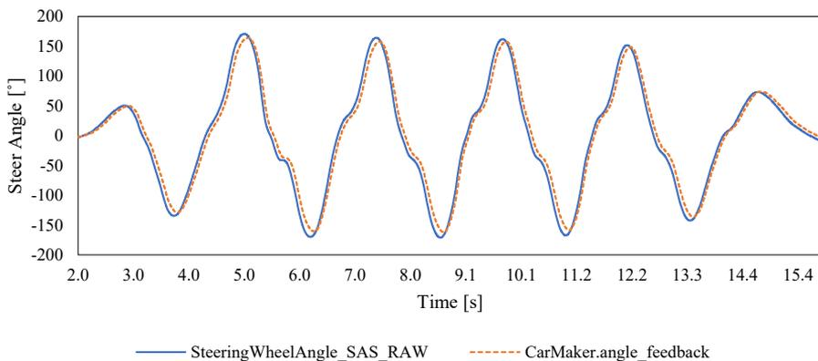
Fig. 12. The steering wheel angle requested by the driver and the angle measured by SAS II.
