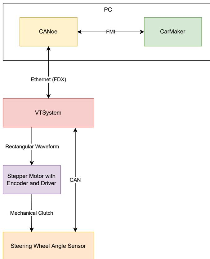
Fig. 3. Testbench diagram including the communication protocols used.
