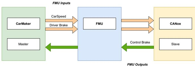
Fig. 5. Scheme of communication between CarMaker and CANoe using FMU in the master-slave architecture.
