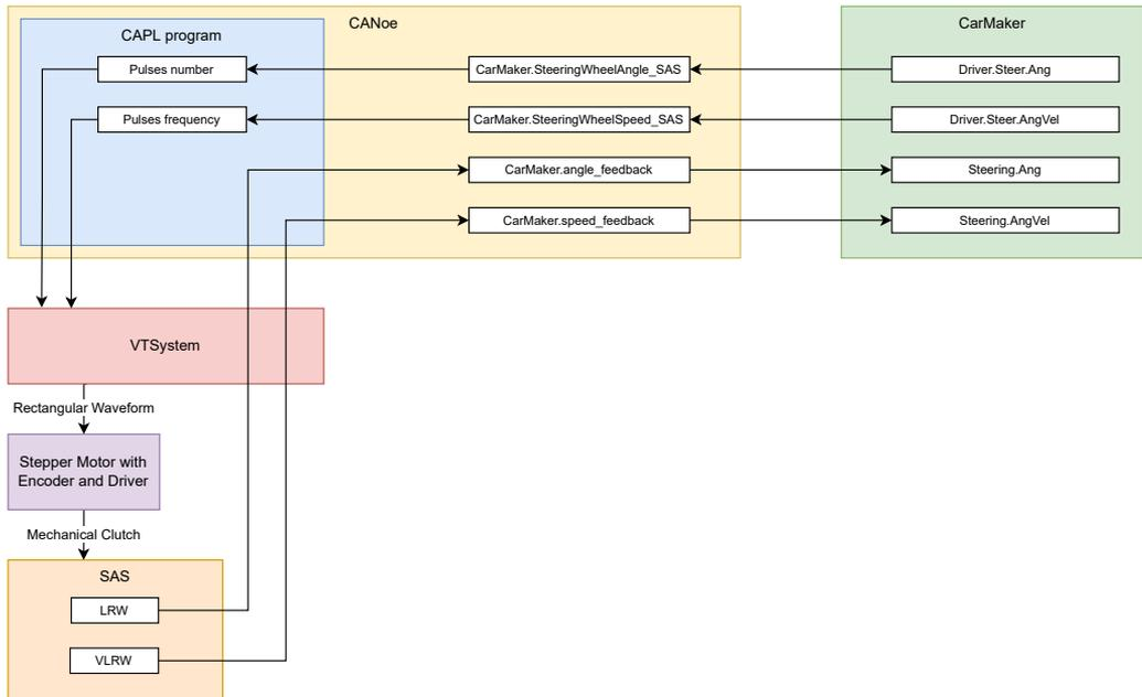
Fig. 7. Flow and mapping of variables between the test system components.
