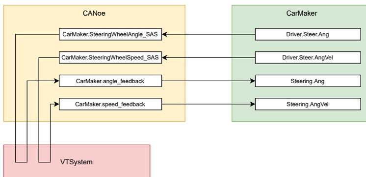
Fig. 8. Devices and variable mapping during determination of errors introduced by the test system.
