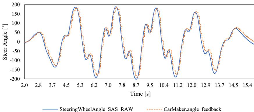
Fig. 10. The steering wheel angle requested by the driver and the angle measured by SAS I.
