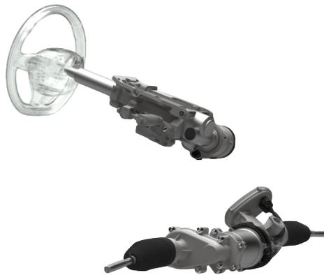
Fig. 1. Steer-By-Wire steering system with visible separation of the steering column from the actuators [3].
