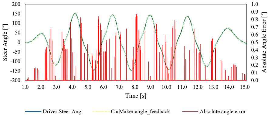
Fig. 9. Superimposed CarMaker transmitted and received angle waveforms and absolute angle error.
