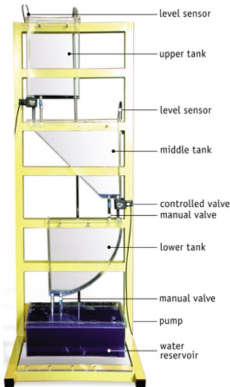
Fig. 1. Multitank system [19]
