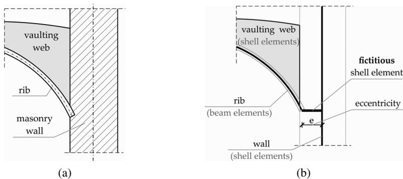
Fig. 4. Modelling of the connection of vaults with walls: a) a sketch illustrating how the loads are transferred from the vaults to the walls; b) sketch of the model of connection of eccentrically oriented shell elements [31]
