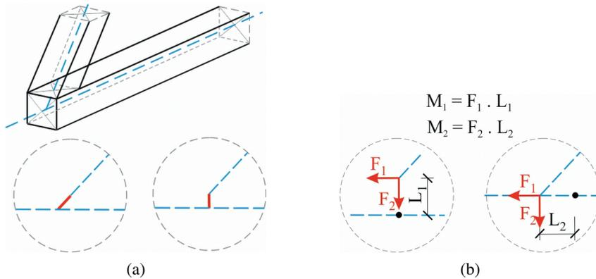
Fig. 2. Modelling of the connection of inclined and horizontal elements of the roof truss [28]:
