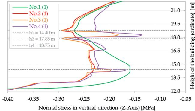
Fig. 12. Normal stresses in the wall in the vertical direction at the height of the connection with the main vault ( $h_4 = 18.75$  m) and the upper support of the side truss ( $h_3 = 17.85$  m) along the line running along the external face of the wall structure (in the axis of the cross-section through the pilaster)
