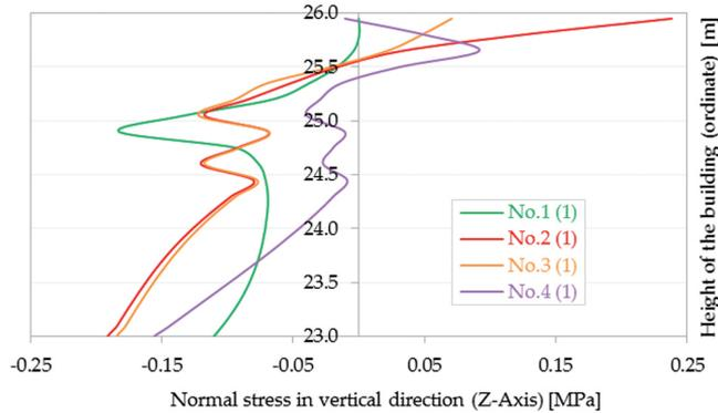
Fig. 11. Normal stresses in the wall in the vertical direction at the height of the connection with the roof truss ( $h_5 = 25.95$  m) along the line running along the external face of the wall structure (in the axis of the cross-section through the pilaster)
