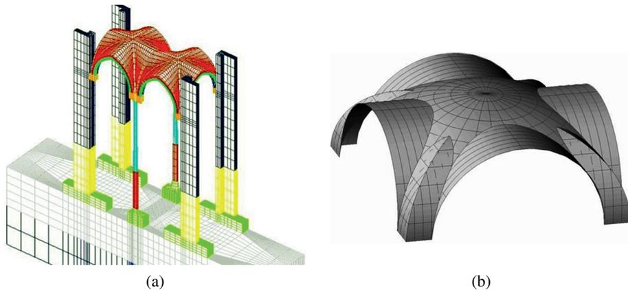
Fig. 3. Examples of modelling of vaults of historic masonry objects: a) a model with the cooperation of vaults with walls [34], b) model of the vault separated from the structure and considered independently [33]
