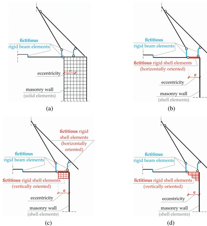
Fig. 7. Static schemes of the connection of the nave's roof truss with the walls and the rigid fictitious elements used in the models: a) reference solid model No. 1, b) model No. 2, c) model No. 3, d) model No. 4
