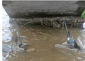
(b) Horizontal displacement measurement
