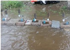
(a) Vertical displacement measurement
