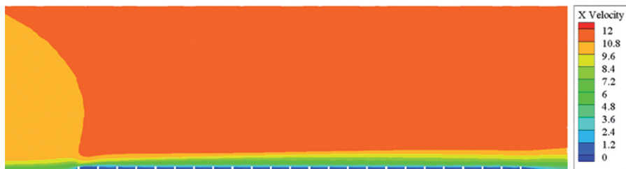
Fig. 10. Cloud map of wind speed around the grass checkered sand barrier
