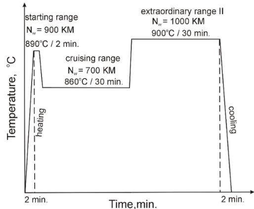
Fig. 2. Diagram of the basic high temperature cycle with a pronounced extraordinary range II of the equivalent durability test of an aircraft engine PZL-10W and the values of power at the main engine shaft corresponding to its individual stages,  $N_w$  and the values of the internal temperature of the engine combustion chamber glow tube
