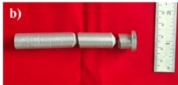
Fig. 2. Specimens a) as cast and extruded specimens & b) Cracked Al-10wt.% of \text{TiB}_2 billet
