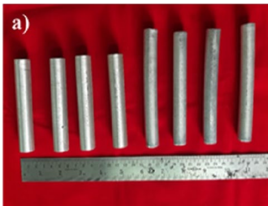
Fig. 2. Specimens a) as cast and extruded specimens & b) Cracked Al-10wt.% of \text{TiB}_2 billet
