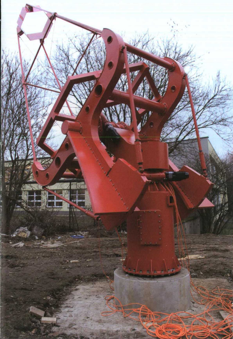
Prototype of the mechanical structure for the small CTA telescope
