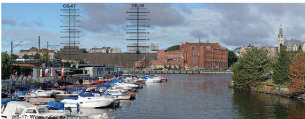
III. 9. Simulation of development at Tobrucki Square (right) and Zawiszy Square (left). The height rulers allow to select the appropriate height of planned buildings not to obscure important elements of the historical city structure or weaken their status in space. By the authors.
