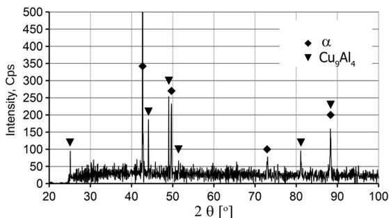
**Fig. 5.** Powder diffraction spectrum defining phases present in the material, Cu–Al solid solution  $\alpha$  and  $\gamma_1$  phase ( $\text{Cu}_9\text{Al}_4$ )
