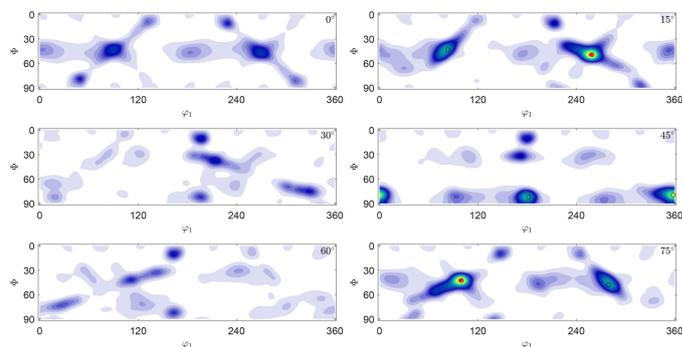
**Fig. 15.** ODF representation of orientation measured for  $\gamma_1$  phase in a sample from zone 3 of DS rod; it corresponds to Fig. 13
