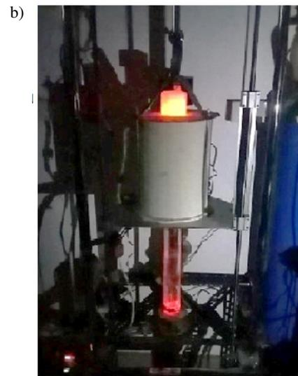
**Fig. 3.** Furnace for directional solidification a) schematic diagram, b) image of real equipment
