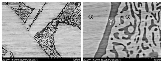
**Fig. 8.** Microstructure of a sample taken from zone III of DS rod; SEM observed using BSE detector; magnifications  $500\times$  and  $5000\times$
