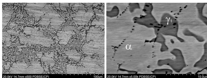
**Fig. 6.** Microstructure of a sample taken from zone I of DS rod; SEM observed using BSE detector; magnifications  $500\times$  and  $5000\times$
