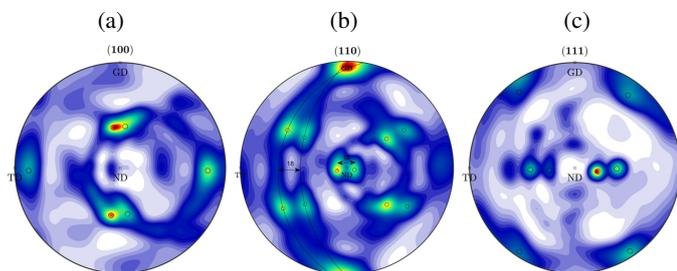
**Fig. 12.** Pole figures of sample from zone 3 of DS rod measured for  $\alpha$  phase at three crystallographic planes  $\{100\}$ ,  $\{110\}$ ,  $\{111\}$  and recalculated in MTEX toolbox for Matlab
