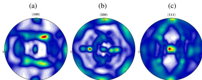
**Fig. 13.** Pole figures of sample from zone 3 of DS rod measured for  $\gamma_1$  phase at three crystallographic planes  $\{100\}$ ,  $\{330\}$ ,  $\{111\}$  and recalculated in MTEX toolbox for Matlab
