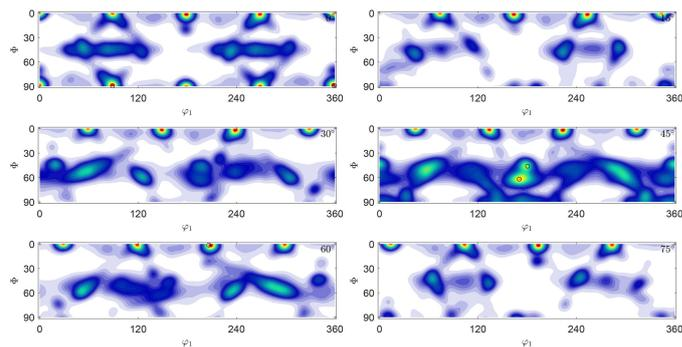
**Fig. 14.** ODF representation of orientation measured for  $\alpha$  phase in a sample from zone 3 of DS rod; it corresponds to Fig. 12
