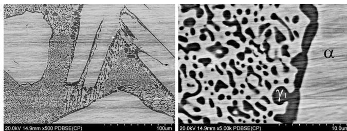
**Fig. 7.** Microstructure of a sample taken from zone II of DS rod; SEM observed using BSE detector; magnifications  $500\times$  and  $5000\times$
