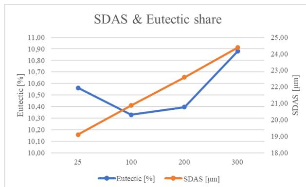
Fig. 6 Comparison of SDAS parameter values and the amount of eutectic in the graph
