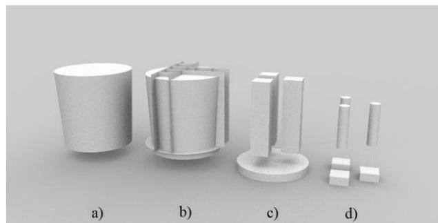
Fig. 1. a) Experimental casting, b) sample splitting, c) sample for spectral analysis and blank for dilatometry, d) samples for metallography, microhardness and rollers for dilatometric measurements
