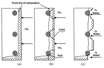
Fig. 2. Stages of destruction of reinforced concrete structure due to carbonation [8]
