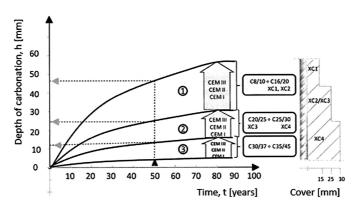
Fig. 3. Required thickness of lagging due to approximate extent of carbonation resulting from concrete strength class and cement type [8,9]
