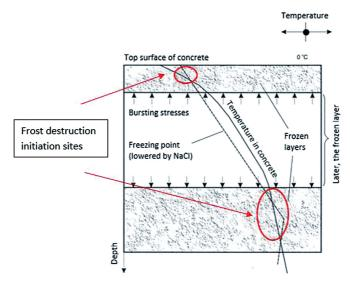
Fig. 4. Frost corrosion mechanism of concrete slab in the presence of de-icing salts (based on [7])
