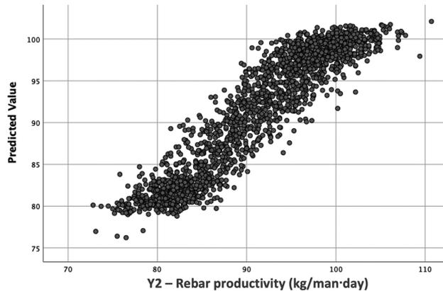
Fig. 11. Comparison chart between predicted and actual rebar productivity
