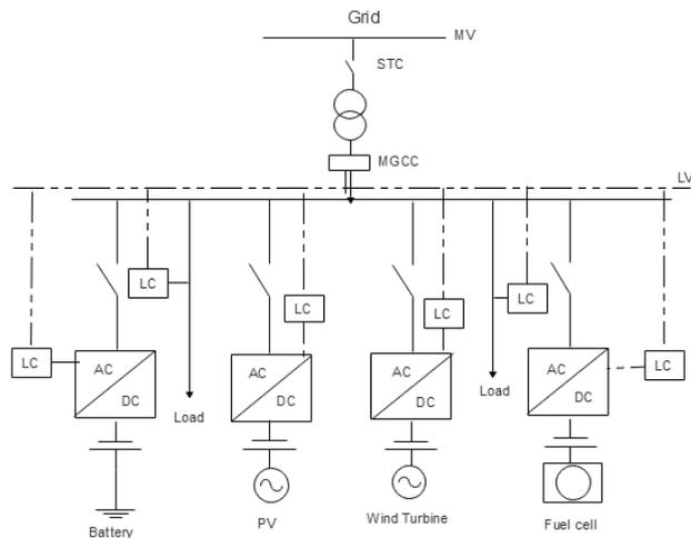
Fig. 2. The structure of the adopted MG system
