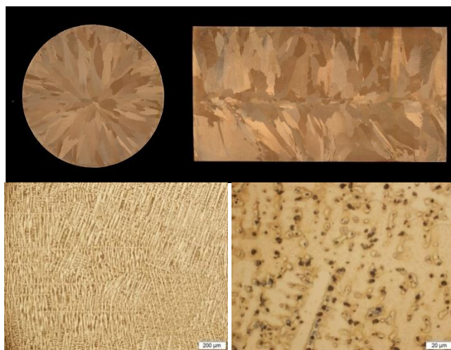
Fig. 7. Macro- and microstructure of cast rod ø22 mm
