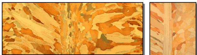
Fig. 8. Structure of the Cu-0.1Ag rod, a/ non-axial, longitudinal section showing *structural zones*: *C*, *C+E*, and *E*, b/ axial, longitudinal section revealing: *C+E*, *E*, and *SC* - *structural zones*; (image, due to courtesy of the Copper Smelter "Cedynia" - KGHM Polska Miedź S.A.)
