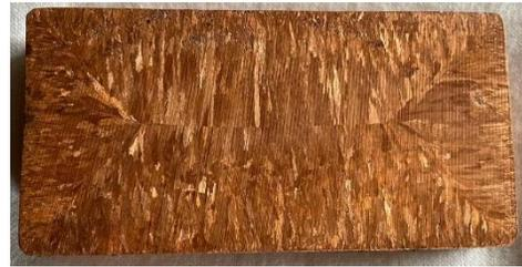
Fig. 1d. Cu-0.1Ag strand 60mm x 120 mm in the cross-section; Contirod – technology; *C* – structure revealed, exclusively.
