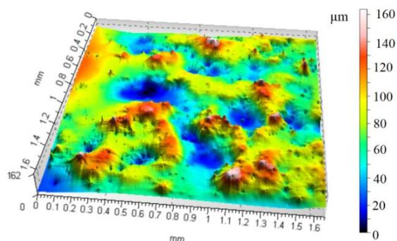
Fig. 9. Isometric view of the surface after EDM at high energy density resulting in large craters
