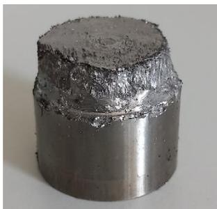
Fig. 1. Typical defects observed in the machining of Alnico alloys
