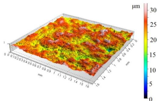
Fig. 8. Isometric view of the surface after EDM at low energy density resulting in low surface roughness
