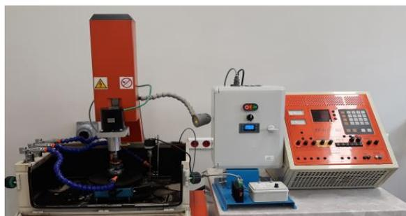
Fig. 2. A system providing additional rotary movements of the tool and the workpiece
