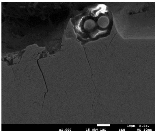
Fig. 11. SEM micrograph of the area adjacent to the cutting zone; EDM at high energy density.
