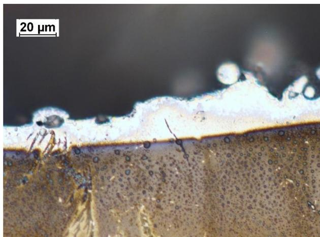
Fig. 12. Structure of the EDM machined Alnico alloy revealed through metallographic examination
