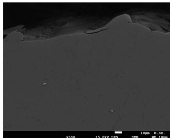
Fig. 10. SEM micrograph of the area adjacent to the cutting zone; EDM at low energy density
