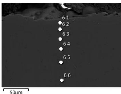
Fig. 7. Measurement points to analyze the chemical composition of the Alnico alloy
