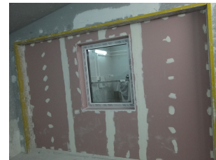
Fig. 4. Sample of the façade installed in the laboratory.
