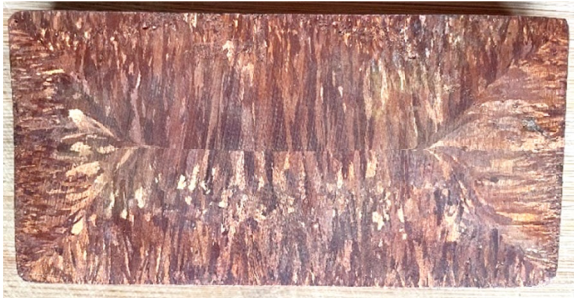
Fig. 1b. Exclusively columnar structure revealed within the copper strand (120 mm × 60 mm); source: KGHM Polska Miedź S.A. – Copper Smelter “Cedynia”
