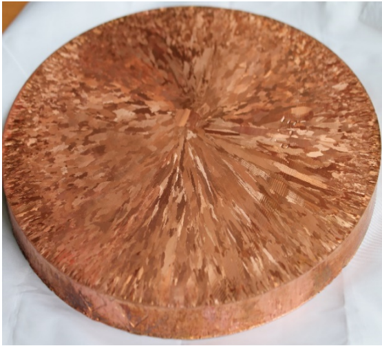
Fig. 1a. Columnar structure revealed within the oxygen-free copper ingot / slice (295 mm in diameter); source: KGHM Polska Miedź S.A. – Copper Smelter “Legnica”
