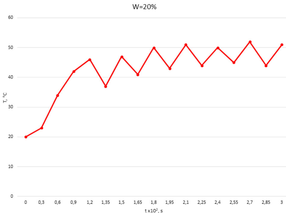
Fig. 5. The change in the temperature of rapeseed having 20% moisture content under 400 W power of microwave energy and the blowing period of 15 s
