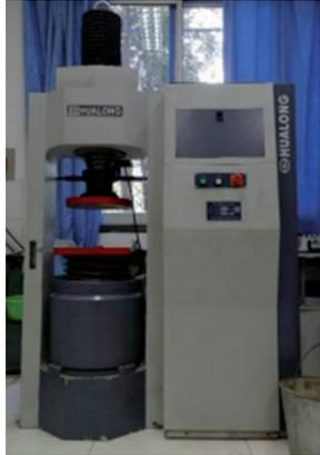
Fig. 2. Uniaxial compression testing machine
