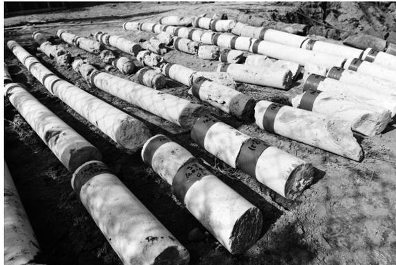
Fig. 6. Core samples of jet grouted material from trial field in Bojszow Nowe [19]
