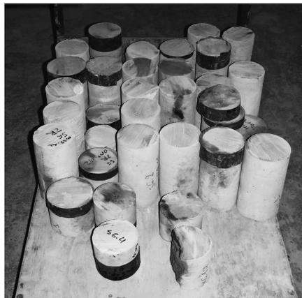
Fig. 8. Cylindrical samples of jet grouted material prepared for uniaxial compressive tests [19]
