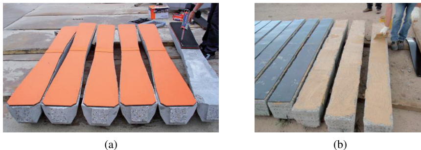
Fig. 9. USPs glued to the bottom surface of the supports: (a) prestressed concrete sleepers [26]; (b) turnout bearers [21]
