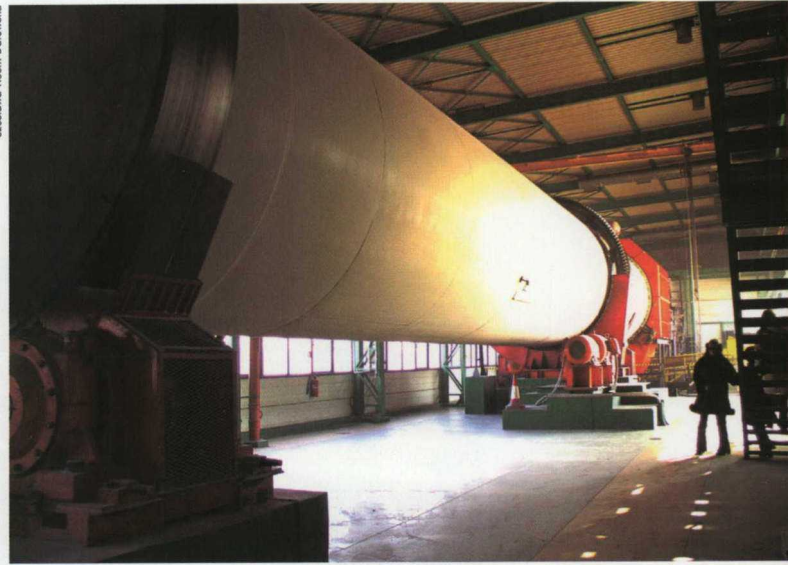
A bioreactor for composting mixed organic waste using the MUT Dano technology
