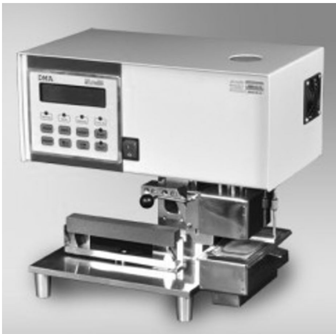
Fig. 1. Universal apparatus for studying hot-distortion phenomena and bending strength, produced by Multiserw-Morek Company [10]
