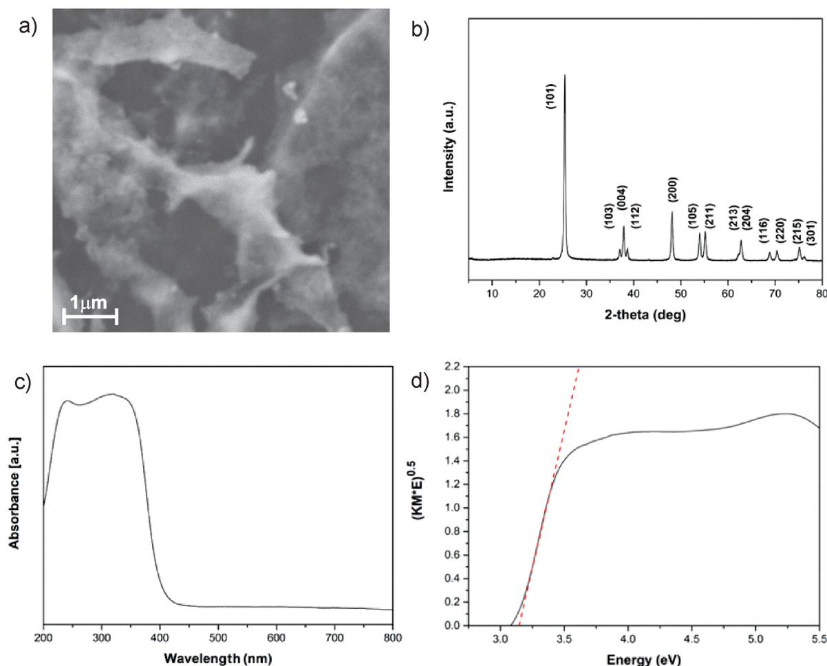
Figure 1. SEM image of 2D TiO<sub>2</sub> photocatalyst (a), XRD pattern for 2D TiO<sub>2</sub> (b), DRS UV-Vis plot of 2D TiO<sub>2</sub> (c) and Kubelka–Munk plot for 2D TiO<sub>2</sub> (d).
