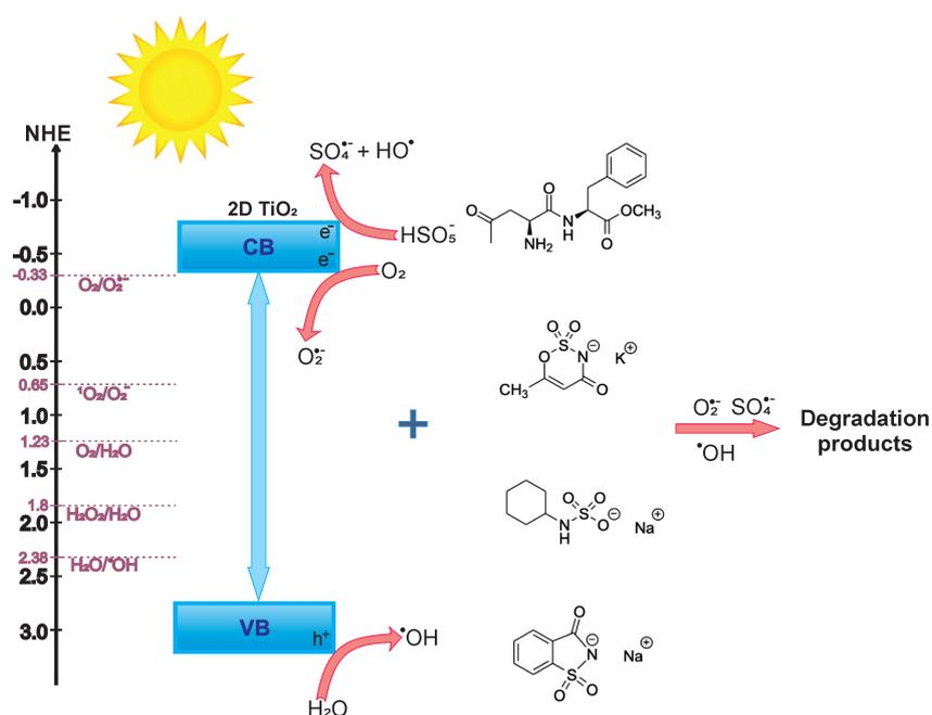
Figure 5. Proposed mechanism of PMS activation over TiO<sub>2</sub> nanosheets.
