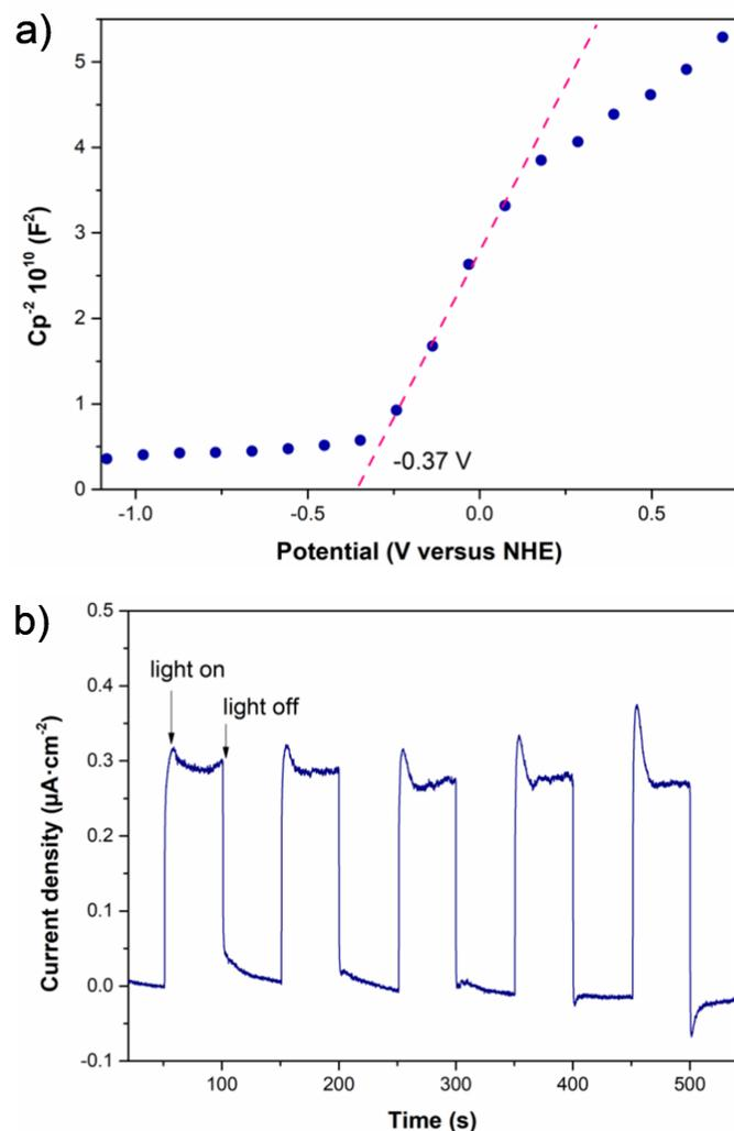
Figure 2. The Mott–Schottky plot for 2D TiO<sub>2</sub> (a), the transient photocurrent response curve of 2D TiO<sub>2</sub> (b).
